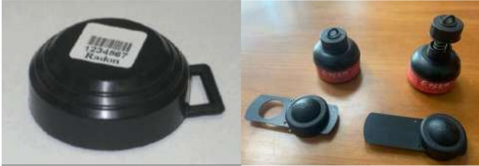
**Figura 8.** Radon-specific passive detector.
